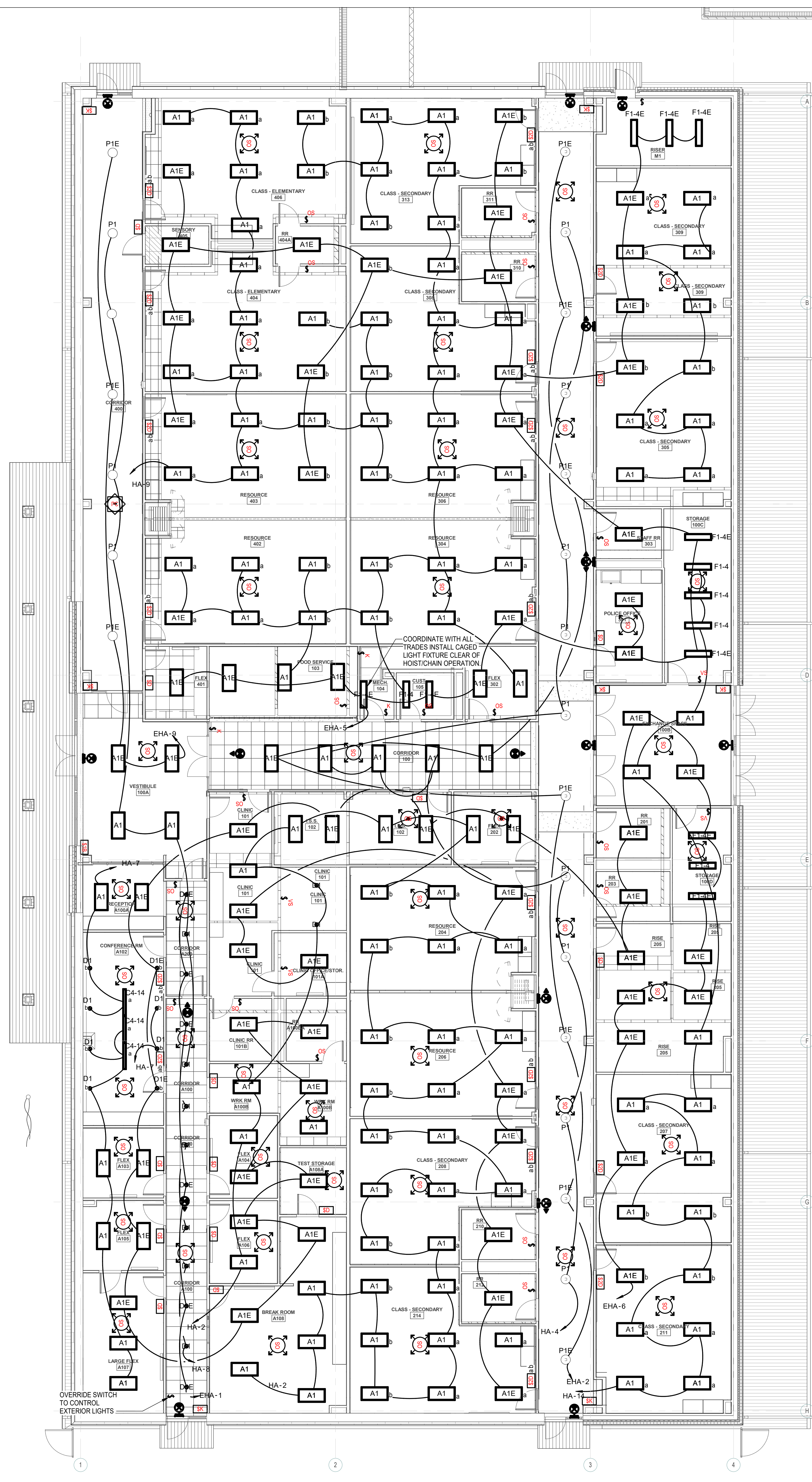
1 ELECTRICAL LIGHTING LEVEL ONE CEILING PLAN SCALE= 1/8" = 1'-0"
