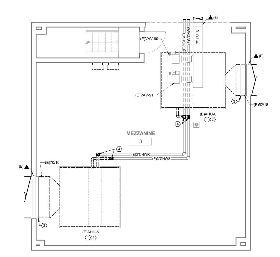
MECHANICAL DEMO ENLARGED PLAN - MEZZANINE 3
