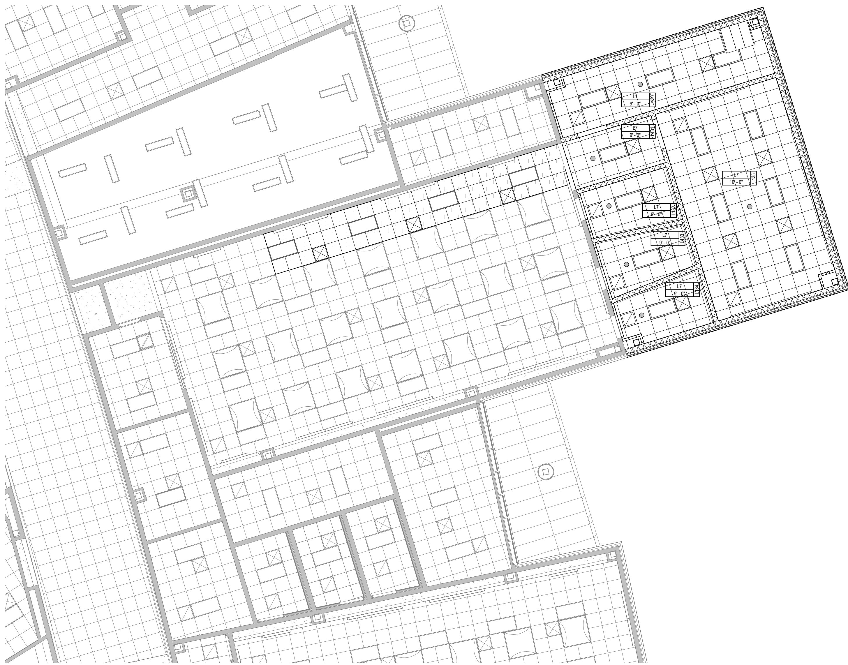
3 AREA L1 - REFLECTED CEILING PLAN 1/8" = 1'-0"
