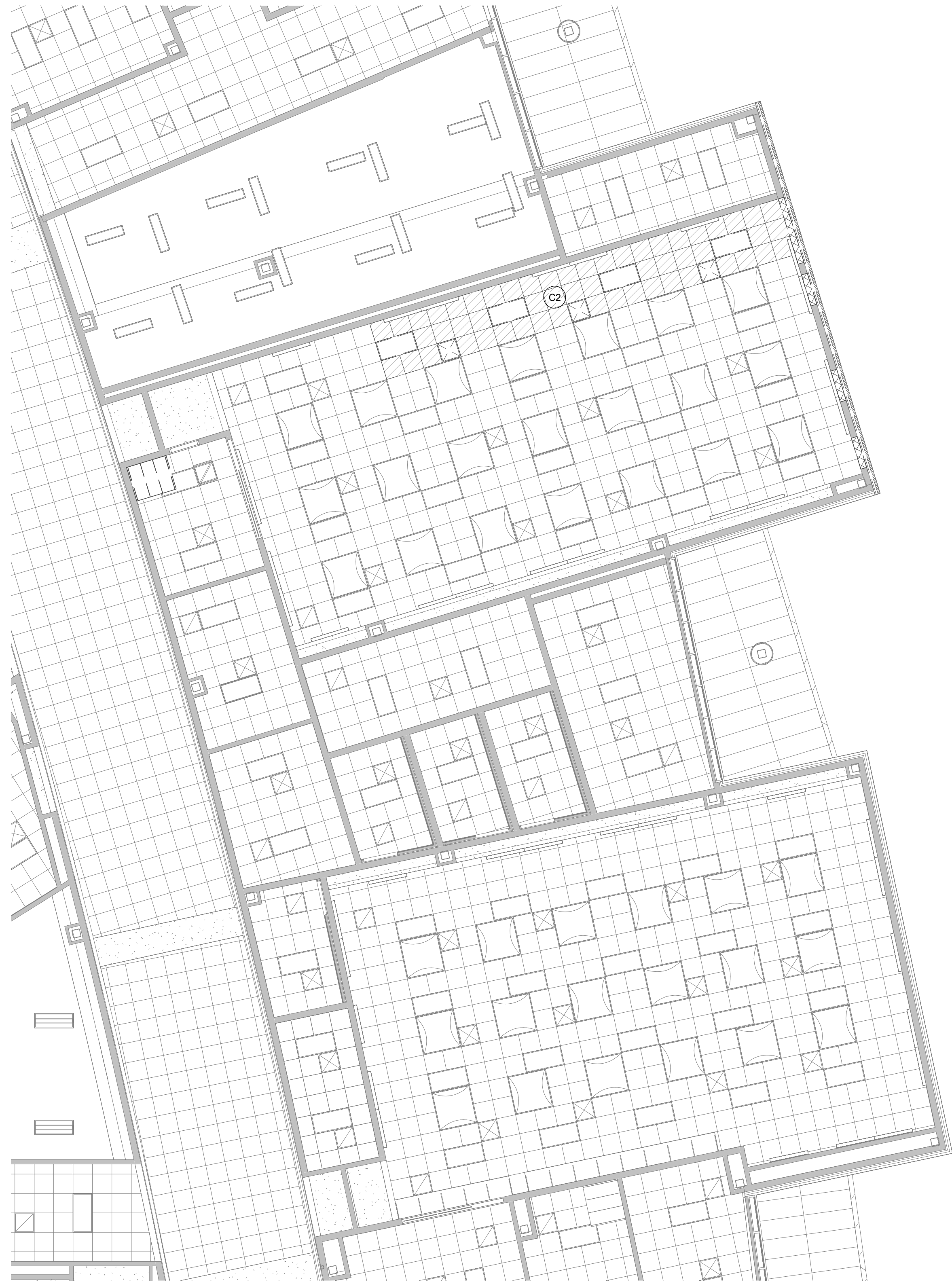
3 AREA L1 - 1ST FLOOR DEMOLITION RCP 1/8" = 1'-0"
