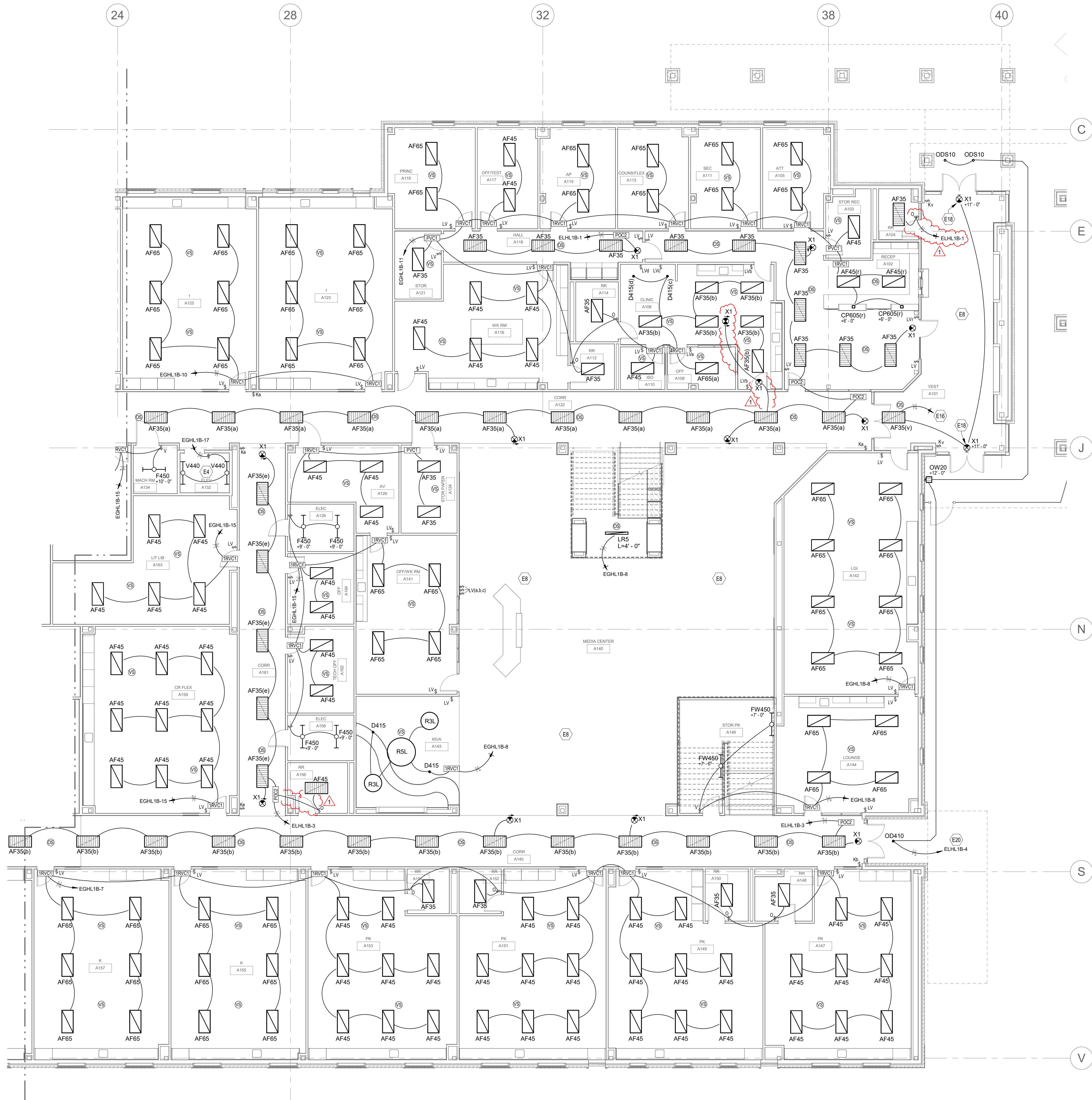
1 ELECTRICAL PLAN - LIGHTING - LEVEL 1 AREA - A1 1/8" = 1'-0"
