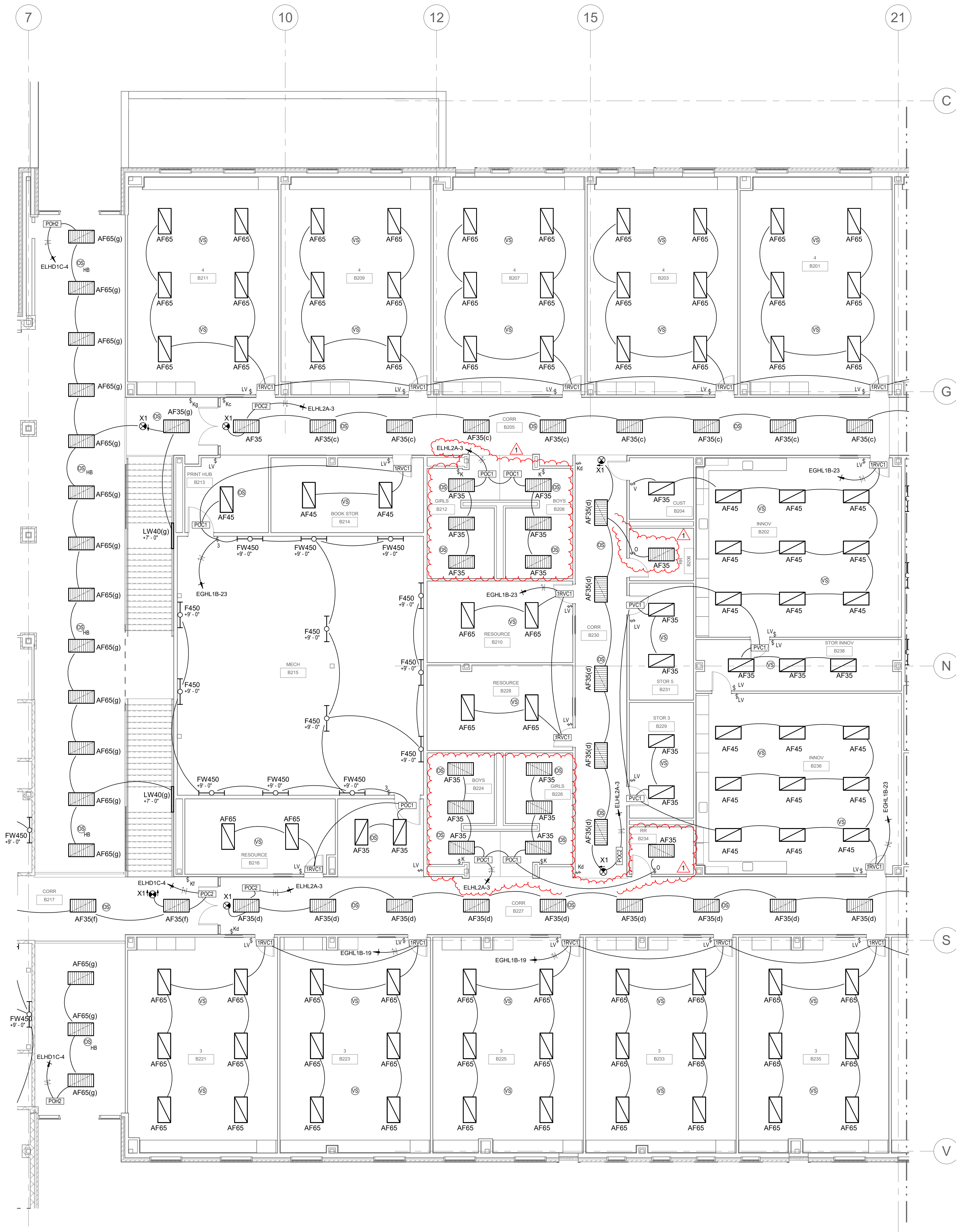
1 ELECTRICAL PLAN - LIGHTING - LEVEL 2 AREA - B2 1/8" = 1'-0"
