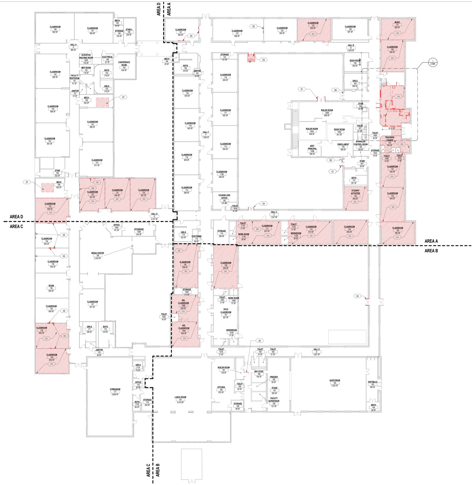
1 DEMOLITION FLOOR PLAN - LEVEL 1
